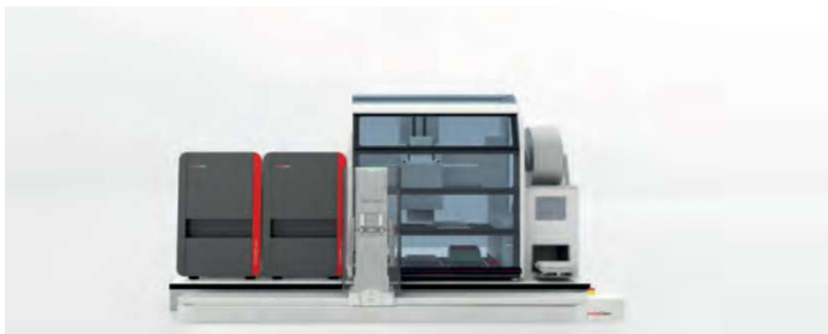
Figure 5 – Example of a fully integrated qPCR workstation. The workstation contains a CyBio®FeliX for preparing qPCR reactions, a CyBio®Carry transport system and 2 qTower Auto automated qPCR thermocyclers. The workstation can be loaded with reagents and left to prepare and run qPCR reactions without user intervention
