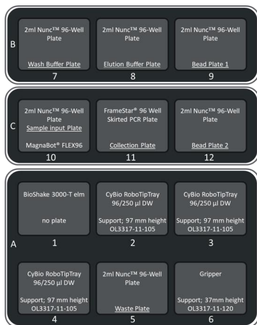
Figure 2. Deck setup for ProNex® Size-Selection Purification System on the CyBio FeliX Liquid Handler. Part 2: Addition of input samples and size selection - (46-57min). Schematic representation (left) and photo (right) of the deck setup for the part 2. The following reagents are dispensed by the user in the selected working wells of 2ml Nunc™ 96-Well Polypropylene DeepWell™ Storage Plates: Wash Buffer at position 7, Elution Buffer at position 8, Sample input at position 10 on the MagnaBot® FLEX 96 Magnetic Separation Device. Position 12 can be left empty for single size selection.
