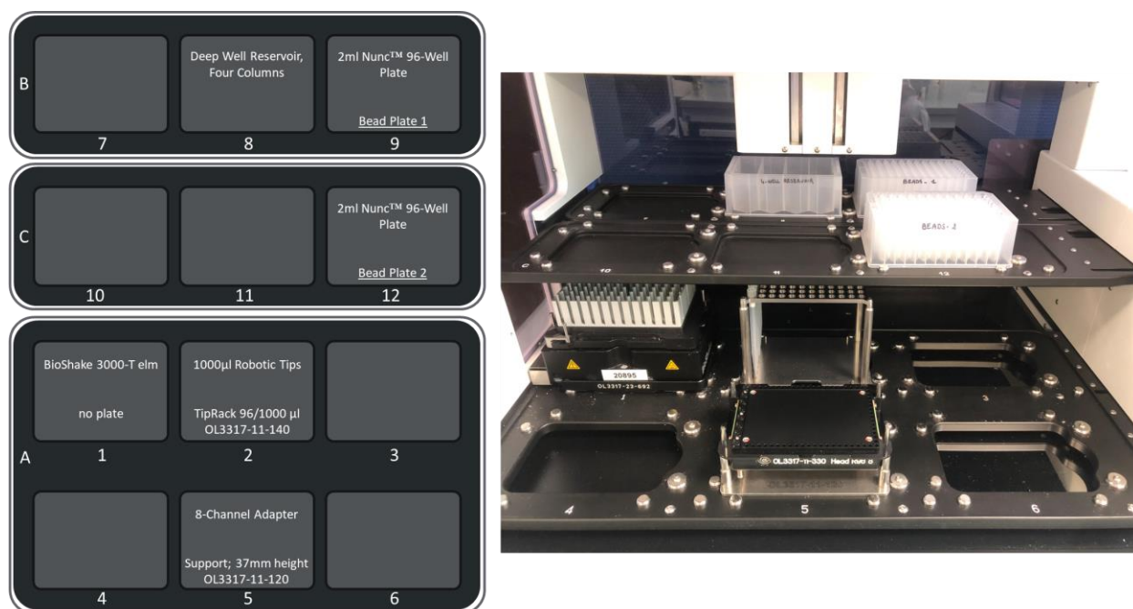
Figure 1. Deck setup for ProNex® Size-Selection Purification System on the CyBio FeliX Liquid Handler. Part 1: Addition of ProNex® Size-Selective Chemistry to the wells of the Bead Plate(s) - (2-5min). Schematic representation (left) and photo (right) of the deck setup for part 1. ProNex® Size-Selection Chemistry (paramagnetic beads) is added by the user to a 4-column Reservoir at deck position 8. The instrument then dispenses the selected volume of beads into the selected wells of a 2ml Nunc™ 96-Well Polypropylene DeepWell™ Storage Plates at position 9 (first size selection) and at position 12 (for dual size selection only, this position can be left empty for single size selection).
