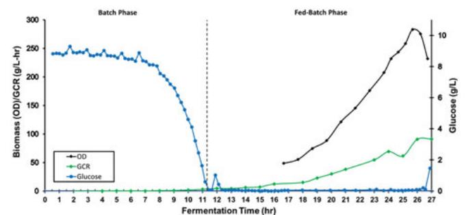
**Figure 3.** Clean Genome *E. coli* Strain B. Real-time media glucose concentration and culture glucose consumption rate data are shown in blue and green, respectively. Culture density is displayed in black. Strain B was cultivated 27 hours to further characterize any process performance limitations.
