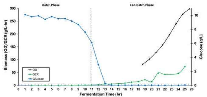
**Figure 2.** Clean Genome *E. coli* Strain A. Real-time media glucose concentration and culture glucose consumption rate data are shown in blue and green, respectively. Culture density is displayed in black. Process duration was 25 hours.
